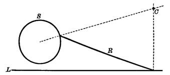
The adjoining figure shows the invariant point (C) when the moving figure is a rigid rod R one end of which slides on a circle S, and the other along a straight line L. This point is the intersection of the radius produced through one end of the rod with the perpendicular to L at the other end.
