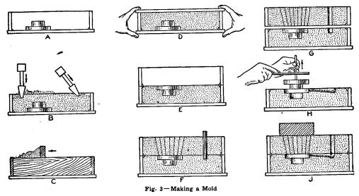
Fig. 3-Making a Mold
