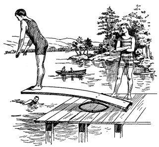
Buggy Springs Used beneath the Board Buggy Springs Used beneath the Board
