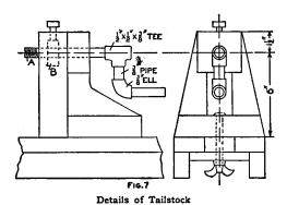
FIG.7 Details of Tailstock
