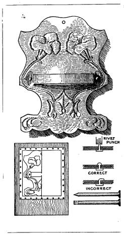
Completed Holder Brass Fastened to Board—Method of Riveting
