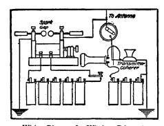
Wiring Diagram for Wireless Telegraph
