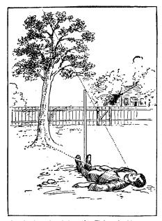
Method of Applying the Triangle Measure
