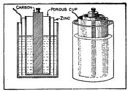
Cross Section and Completed Cell
