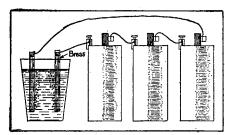
How Wires are Connected
