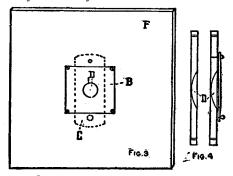
Pin Hole and Shutter Construction
