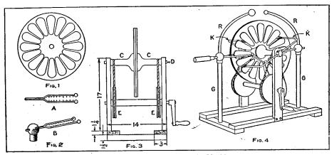
Details of a Homemade Static Machine
