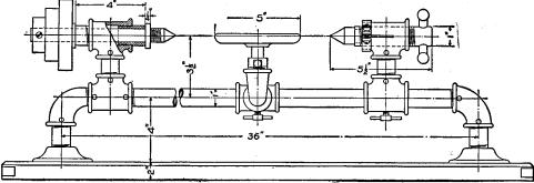
Fig. 1-Details of Lathe
