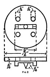
a blacksmith make a crank 8 in. long, threaded for 5 in. as shown. At the dead center end taper the crank and make a cup center, out of which allow a 3/16-in. point to project. The cup prevents the point from boring into
