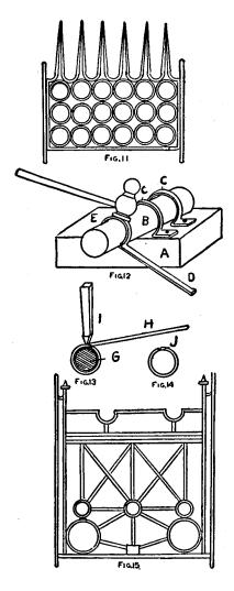
sufficiently stiff by uniting two sides with rivets. The ends at top are looped as shown, while the ends or butts at the base are opened out to make the feet. Rings are shaped on forms and are then riveted to the base cross-piece as illustrated. Crosses are made to describe to central design and the plan is worked out quite readily with the different shapes.
