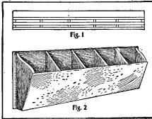
the clothes closet. Figure 1 shows the construction of the bottom to permit the dirt to fall through. Two boards, 9 in. wide and about 3 ft. long, with six partitions between, as shown, will make pockets about 6 in. long. The width of the pockets at the bottom is 2 in. and at the top 5 in.-Contributed by Guy H. Harvey, Mill Valley, Cal.
