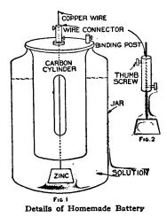
Fig.1 Details of Homemade Battery
