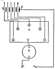
you have the current of one battery; when A is on No. 2 you receive the current from two batteries; when on No. 3, from three batteries; when on No. 4, from four batteries, and when on No. 5, from five batteries. More batteries may be connected to each point of switch B.
