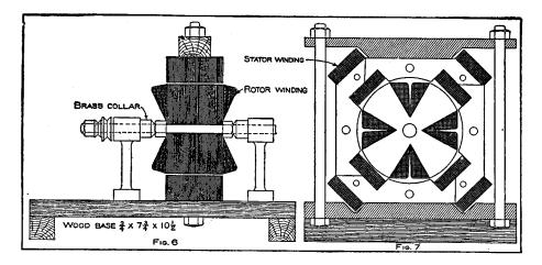
about 2-1/2 lb. being used, and the connections are such as to produce alternate poles--that is, the end of the first coil is joined to the end of the second the beginning of the second to the beginning of the third, and the end of the third to the end of the fourth, while the beginnings
