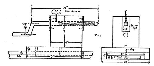
diameter, using longer 3/16-in. stove bolts with heads countersunk. Rotate the lathe, and with a gimlet bore a hole at the exact center and through the board. Now take off the board and countersink on the back a place for the head of a coarse threaded screw. Turn in a 1-3/4 -in. screw, replace the board and any block held on the end of the rotating screw will turn on and be held while being turned. --Contributed by L. L. Winans, Mexico, Mo.
