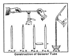
Construction of Geissler Tube
