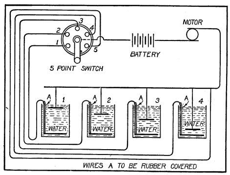
Wiring Plan for Water Rheostat
