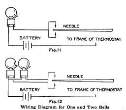
Wiring Diagram for One and Two Bells
