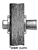
The work of finishing a number of brass castings with flat sides was accomplished on an ordinary polishing wheel, from which the first few layers of cloth were removed and replaced with emery cloth. The emery surface of the cloth was placed outward and trimmed to the same diameter as the wheel. This made a sanding and polishing wheel in one. --Contributed by Chester L. Cobb, Portland, Maine.
