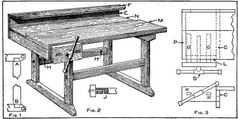
Details of Construction of Homemade Workbench
