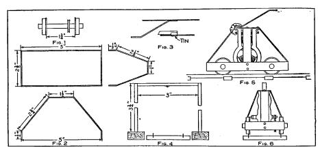
The Different Parts for Making the Electric Locomotive
