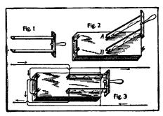
Simple Current-Reversing Switch Simple Current-Reversing Switch
