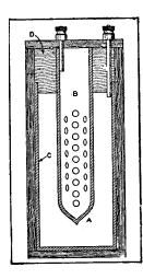
as possible, except for about 1 in. on each end. One end of this tube is hammered together as shown at A in the sketch to make a pocket to hold the paste. This, of course, does not need to be watertight.
