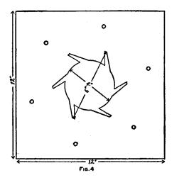
Now take another of the 12-in. square pieces of wood, and cut it out as shown in Fig. 4, slightly beveled. After it is finished, place it between two of the 12-in. square pieces of wood, one of which should have a 3/8-in. hole bored through its center. Then bolt together with six 1/4-in. bolts, as shown by the
