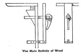
and the excess taken up on the other end by an eccentric lever. The wedge is worked by a string passing through the top of the bench and should be weighted on the other end to facilitate the automatic downward movement.
