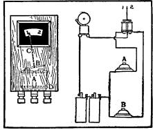
Annunciator and Wiring Diagram
