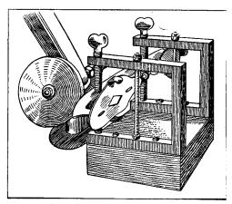
Skate Runner Fastened in Clamp Skate Runner Fastened in Clamp
