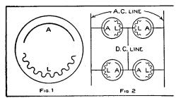
Electrolytic Rectifier and Connections
