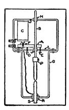
the top and 4 in. at the bottom. A cross bar, L, made of the same material, is fitted into the off-set in the frame and riveted. Holes are drilled through the frame and brass bushings, H and J, are fitted for bearings to receive the adjusting brass rod, B, which should be 1/4 in. in diameter. A brass curtain rod can be used for the rod B, and on its lower end a socket, P, is soldered.
