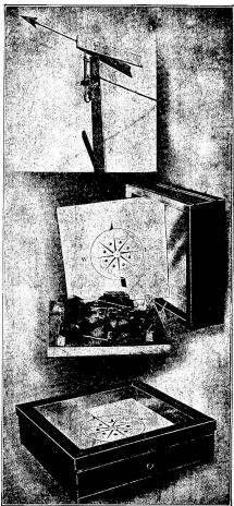
The Wind Vane, Magnets and Indicator
