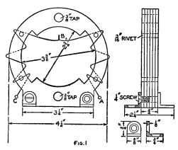
The Field-Coil Core is Built Up of Laminated Wrought Iron Riveted Together
