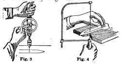
Drilling and Sawing the Metal
