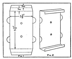
Pattern for Cutting the Metal Pattern for Cutting the Metal
