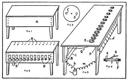
How the Electric Piano is Constructed
