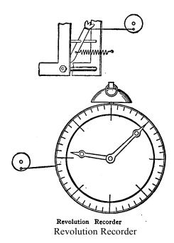
unwound the hour hand starts on a new trip. The clock I used was put on an amateur windmill and when the hour hand went around once 86,400 revolutions or jerks on the wire were made, while the minute hand recorded one-twelfth of this number, or 7,200. -- Contributed by Richard H. Ranger, Indianapolis, Ind.
