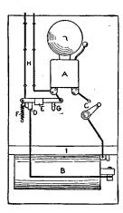
1 in. long to key, then wind the alarm just enough so that the key stands straight up and down. Place the clock on the shelf and the key under the flange of lever E. Pull lever G down out of the way and close the lever on the switch. The alarm key will turn and drop down, letting lever E drop into the V-shaped piece D and make connection.
