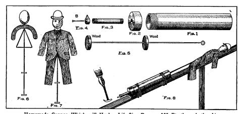
Homemade Cannon Which will Hurl a Life-Size Dummy 100 Ft, through the Air Homemade Cannon Which will Hurl a Life-Size Dummy 100 Ft, through the Air
