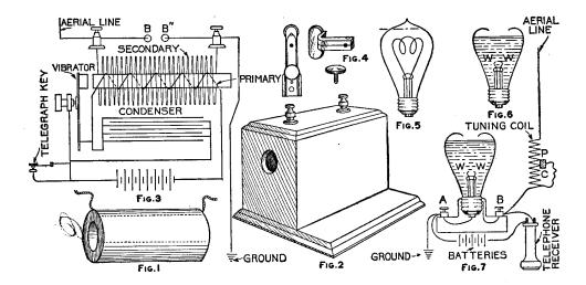
The aerial line, No.6 stranded, is run from binding-post B through the choking or tuning coil, and for best results should extend up 50 ft. in the air. To work a 20-mile distance the line should be 100 or 150 ft. above the ground. A good way is to erect a wooden pole on a house or barn and carry the aerial wire to the top and out to the end of a gaff or arm.
