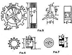
Armature-Ring Core, Its Hub and the Construction of the Commutator and Its Insulation
