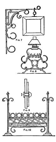
for making these stands, as every part is bent as described in connection with the bending forms, and the portions are simply riveted at the different junctures. Both iron and copper rivets are used as at I, in Fig. 9, a cross sectional view.
