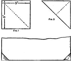
Fig 3 Paper Corners for Blotter Pads
