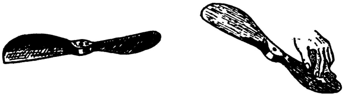
FIG. 43. All carving finished. Sandpapering to secure a smooth surface.
