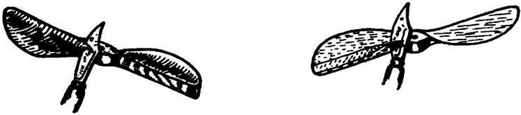
FIG. 42 Rounding the back of the first blade. Rounding the back of the second blade.
