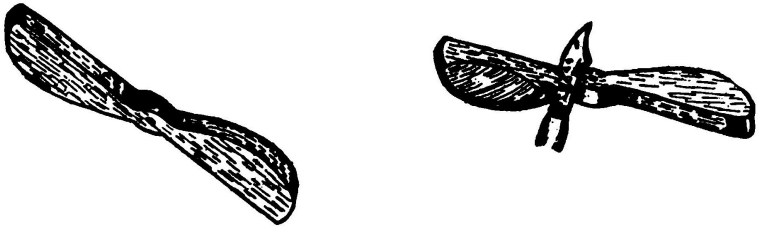
FIG. 40. The first step in carving a propeller. The blank. Hollowing the first blade.
