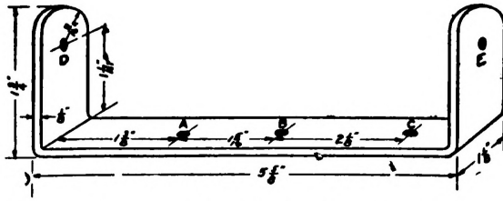
FIG. 146.—Details of the Engine Frame.
