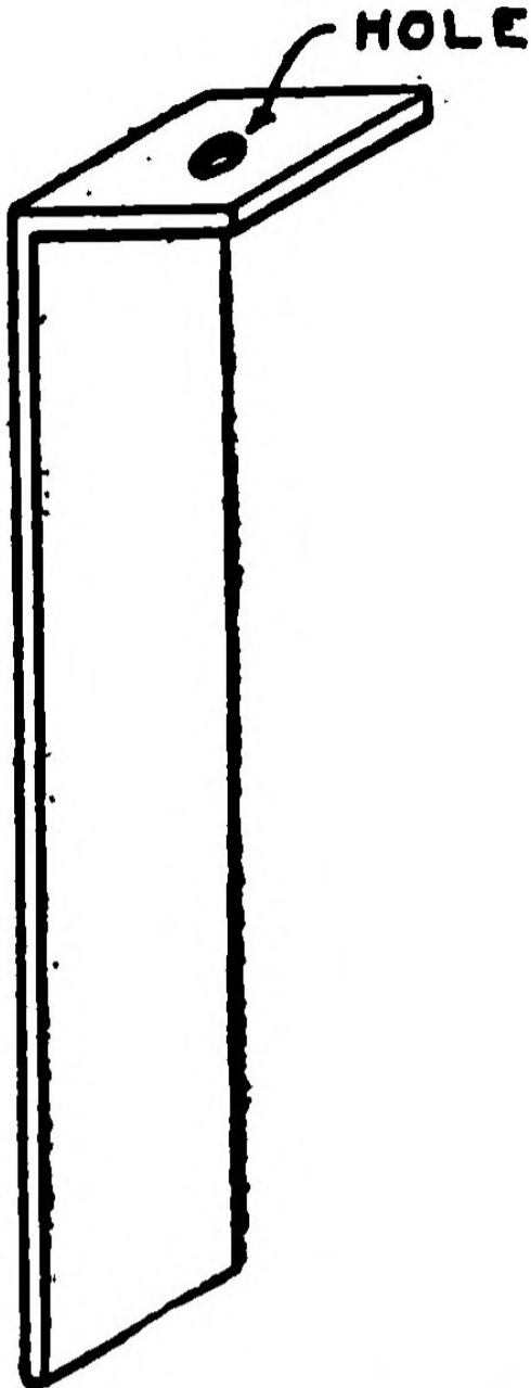
FIG. 50.—An Electrode cut out of Sheet Metal. The top
