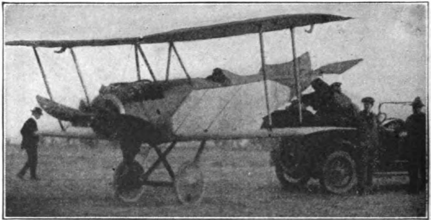
Fig. 1. Curtiss "Baby". Biplane Speed Scout. Equipped with 100 Horsepower Water Cooled Motor.
