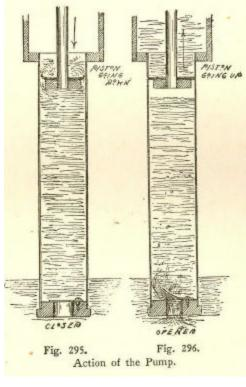
Fig. 295. Fig. 296. Action of the Pump.
