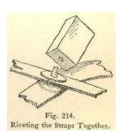
Fig. 214. Riveting the Straps Together.
