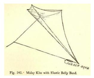
Fig. 242. Malay Kite with Elastic Belly Band.
