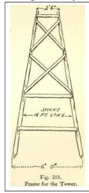
were from 4 to 6 inches in diameter. With them we made two frames of the form given in Fig. 283, using slabs to brace them apart. These frames were now set in position, with their lower ends firmly planted in holes in the ground, and the tower was completed by nailing on a number of diagonal braces. A couple of boards were nailed across the upper ends at opposite sides, and holes were drilled through them to provide bearings for the wind wheel shaft.
