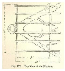
Fig. 139. Top View of the Platform.
