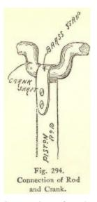
Fig. 294. Connection of Rod and Crank.
