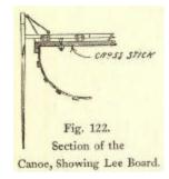
Fig. 122. Section of the Canoe, Showing Lee Board.
