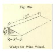
Fig. 286. Wedge for Wind Wheel.
