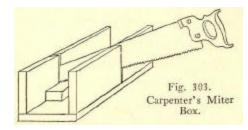
Fig. 303. Carpenter's Miter Box.
