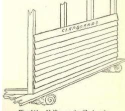
Fig. 141. Nailing on the Clapboards.
