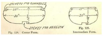
Fig. 124. Center Form. Fig. 125. Intermediate Form.
