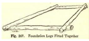
Fig. 267. Foundation Logs Fitted Together.
