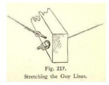
Fig. 217. Stretching the Guy Lines.
