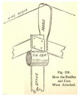
Fig. 258. How the Paddles and Cans Were Attached.
