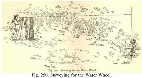
came in line with the eleventh chalk mark. The top of the filter was, therefore, 11 feet above the level of the river. Bill figured that it would be necessary to construct a wheel about 15 feet in diameter in order to raise the water to the proper height.
