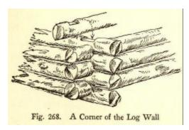
Fig. 268. A Corner of the Log Wall.
