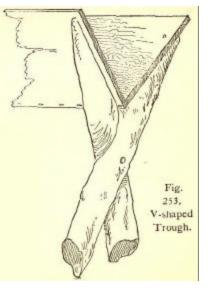
Fig. 253. V Shaped Trough.
