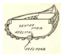
Fig. 128. Section at Center of Canoe.
