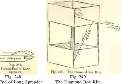
Spreader. Fig. 248. Forked End of Long Spreader.
