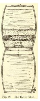
Fig. 69. The Barrel Filter.
