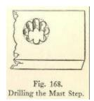
Fig. 168. Drilling the Mast Step.
