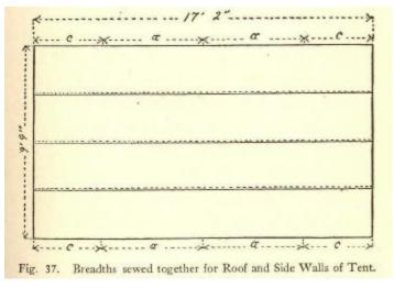
Fig. 37. Breadths sewed together for Roof and Side Walls of Tent.
