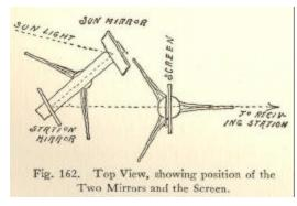
Fig. 162. Top View, showing position of the Two Mirrors and the Screen.
