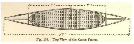
Fig 109. Top View of the Canoe Frame.
