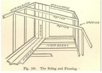
Fig. 184. The Siding and Flooring.
