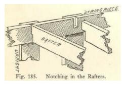
Fig. 185. Notching in the Rafters.
