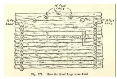
Fig. 271. How the Roof Logs were Laid.
