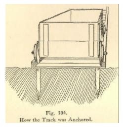
Fig. 304. How the Track was Anchored.
