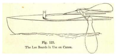
Fig. 123. The Lee Boards in Use on Canoe.
