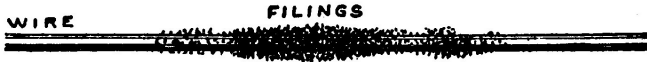
FIG. 1.—If a current of electricity is passed through a wire, the wire will attract to itself iron filings.
