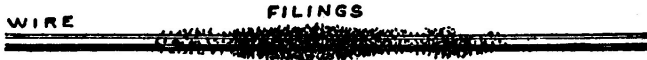
FIG. 1.—If a current of electricity is passed through a wire, the wire will attract to itself iron filings.
