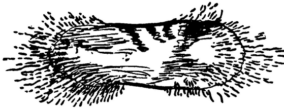
FIG. 1. Lodestone which has been Dipped in Filings to show Poles
